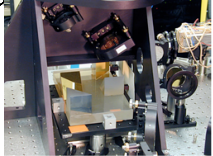
Side view of the periscope assembly of the Achromatic Nulling Testbed.
